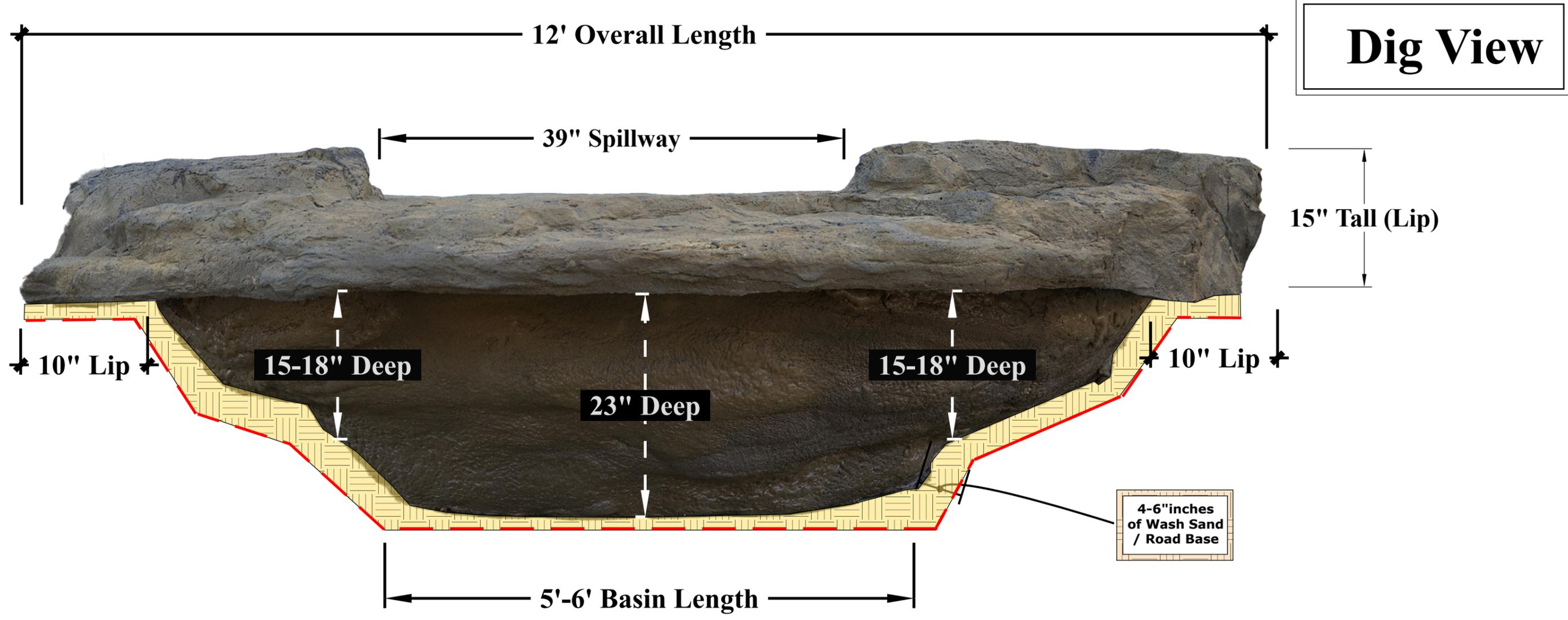
All Measurements under ground must add an additional 4"-6" inches to create space for the 4"-6" inches of WASH sand or Road Based Gravel that will be washed in under the Lagoon Spa in order to create a tight fit for the spa.
